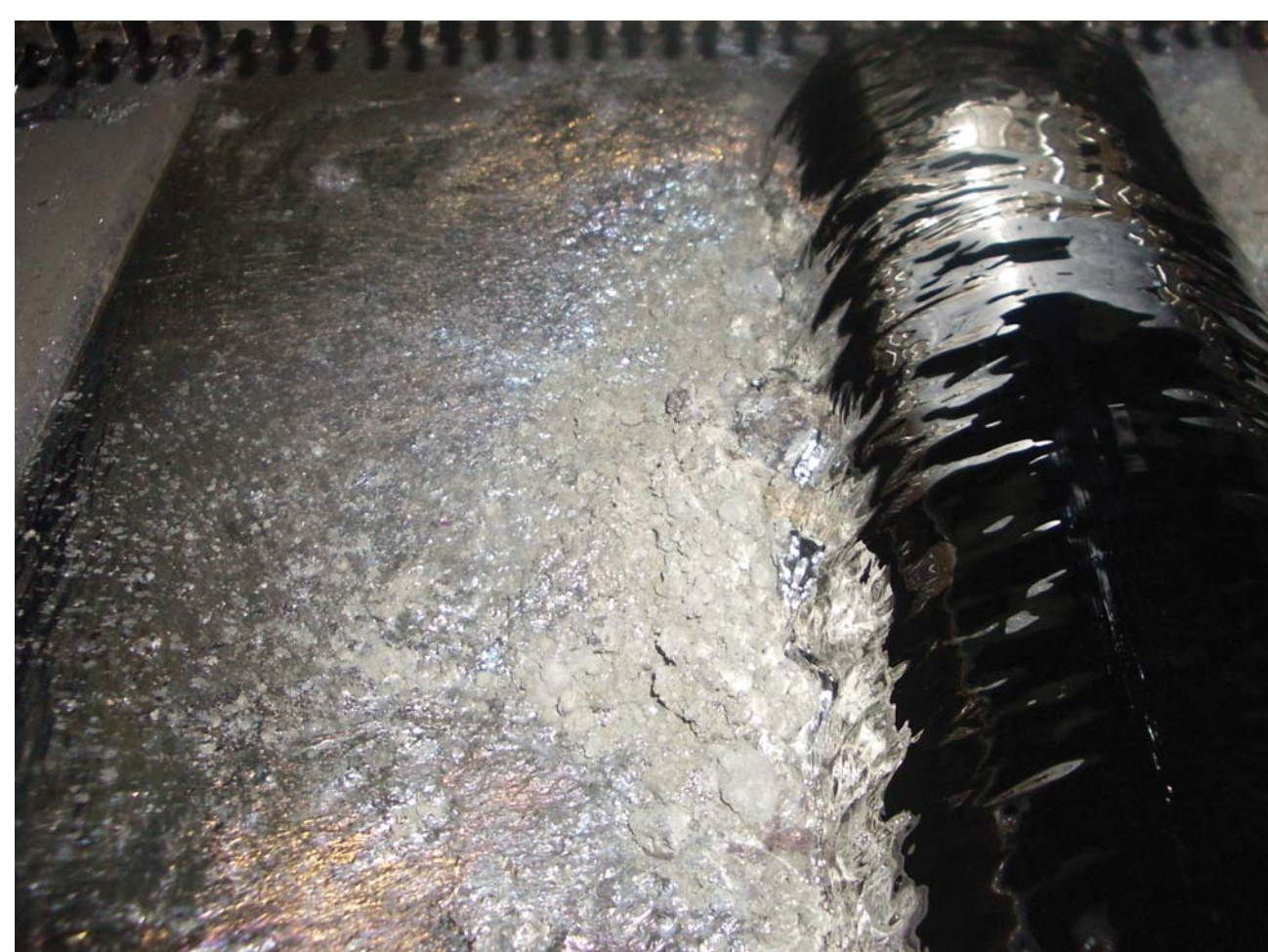
Lead-free solder bath without MS2™, showing typical dross buildup
