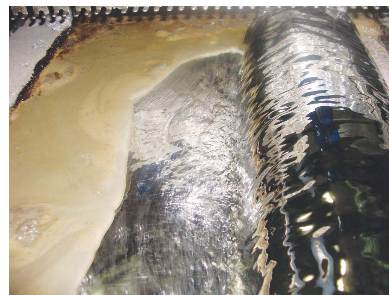
Lead-free solder bath with MS2™, showing no dross—only shiny solder
