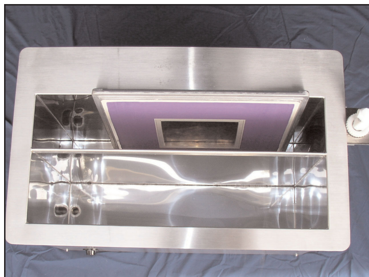
Wash and Rinse Tank Assembly Shown with 23-inch stencil
